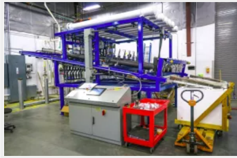
IBHS conducts hail research in the Laboratory Building for Small Tests, where hailstones of various sizes are recreated and propelled against roof samples. Photos: Insurance Institute for Business and Home Safety.
