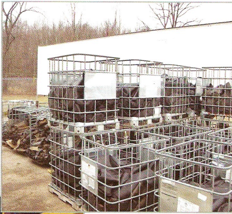
Photos 4, 5, and 6 – Membranes are stacked and stored for transportation to the grinder. (Photos courtesy of WDG).
