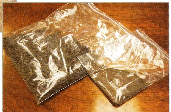
Photos 1, 2, and 3 – EPDM is removed from a ballasted system (above, left). Afterward, it is taken to the grinder (top right), and the final product results (bottom right). (Photos courtesy of ERA.)
