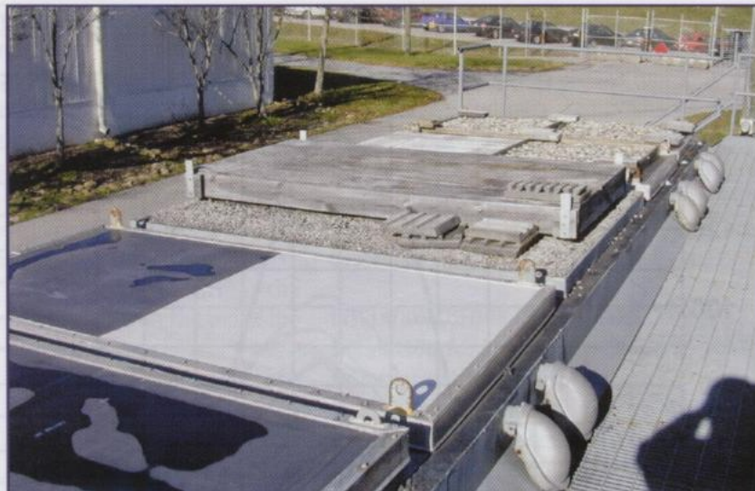
Figure 6 – RTRA configured for ballasted system analysis.
